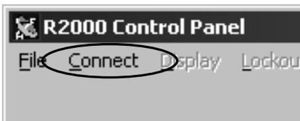
As long as there is a connection between the PC and the Radiometer, data is automatically downloaded to the PC. A 9-pin serial cable is provided with each R2000 Radiometer.
