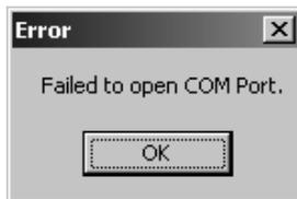
Select from the File pull down menu – COM Ports. Ensure that the applicable COM port is checked and cable is connected to corresponding plug. Try connecting again.
