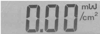
If the display is not showing the " $\text{cm}^2$ ", it indicates that the R2000 Radiometer is in Power mode. Simply press the POWER/IRRAD keypad button to toggle into irradiance mode.
