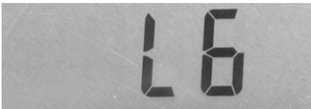
When a light guide is fully inserted the display will clear. If the message remains after the light guide has been inserted try removing the light guide and re-installing it.
