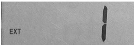
If multiple devices are connected each press of the EXTERNAL keypad button will increment to the next external device before returning back to internal mode.
