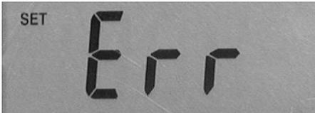
If the **EXT** icon is illuminated on the display with the **Err** message displayed it indicates that the R2000 Radiometer was unable to communicate with an external adapter.
