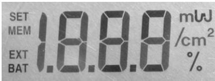
**Note:** If a light guide adapter is installed in the optical port, the display will flash the diameter of the light guide adapter for 3 sec.
