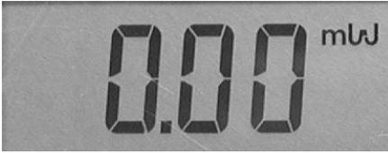
If the display is showing " $\text{m}^2/\text{cm}^2$ ", press the POWER/IRRAD keypad to toggle into Power mode.
